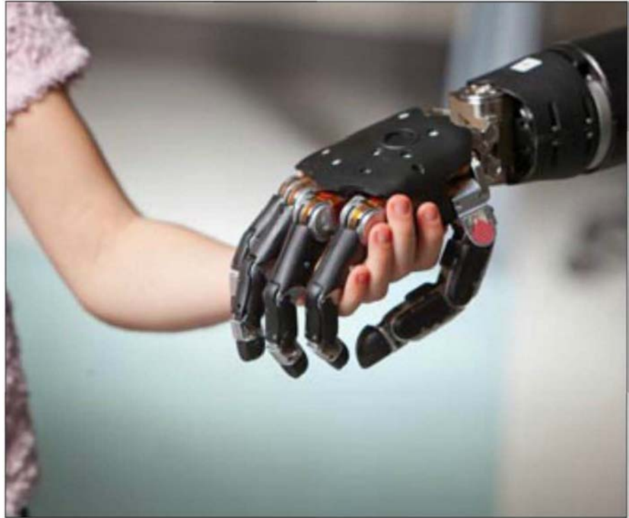
Fig. 3 - Functional prosthetic arm. (Courtesy of the Johns Hopkins University Applied Physics Laboratory)
